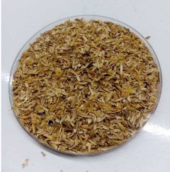
Rice husk coarse mill (40 mesh)
