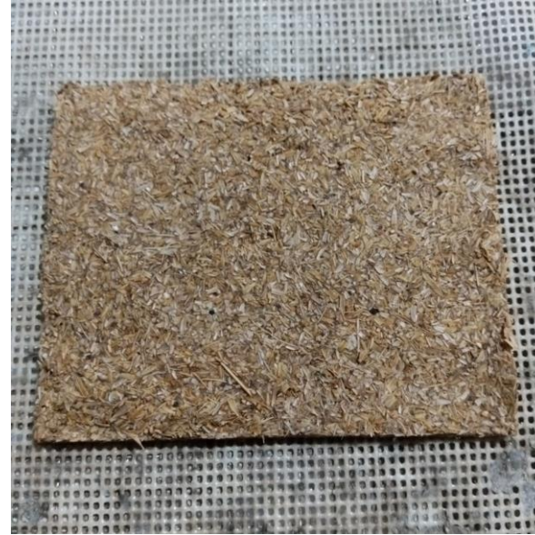
Particle rice husk board (medium mesh)
