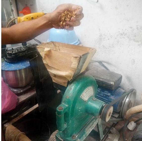
Milling rice husk with Disk mill
