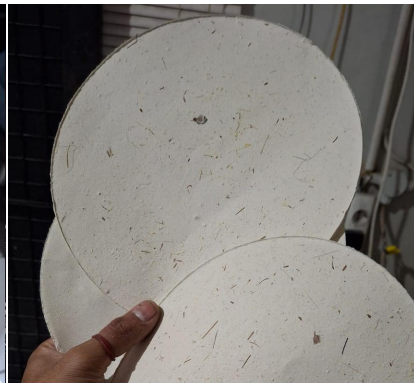
Image.10: Result Of Paper From Rice Straw With Raw Fiber Using Circular Mold Screen
